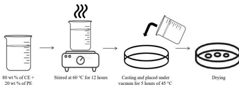
**Figure 1** Methods of preparing the composite electrolytes system.
