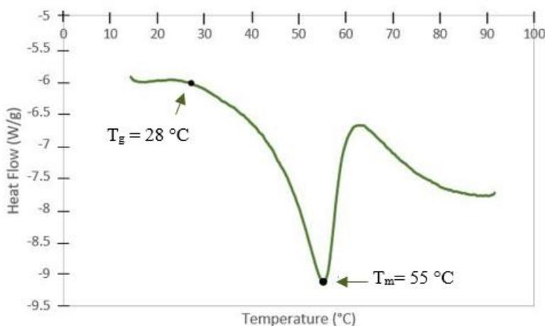
**Figure 4** DSC graph of composite electrolyte sample.
