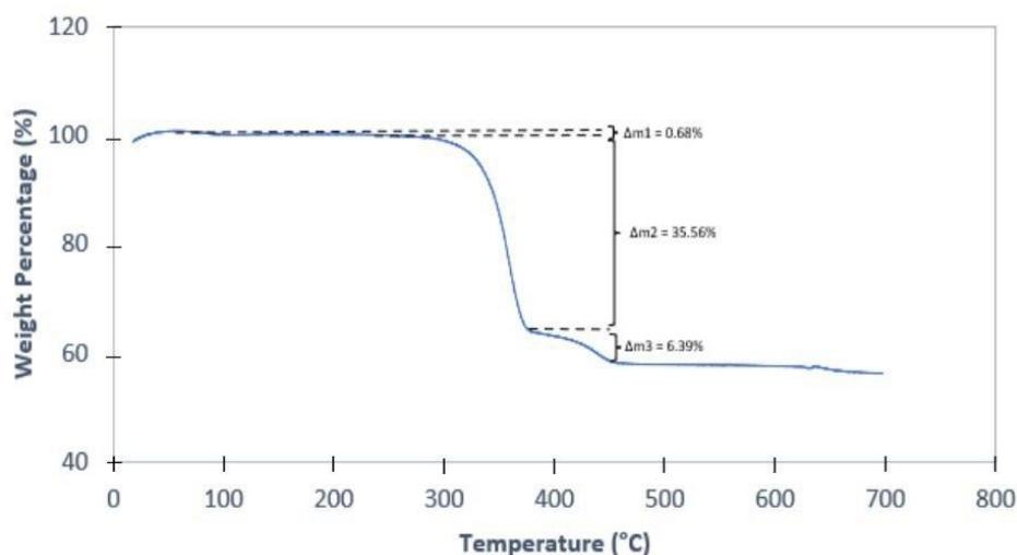
**Figure 3** TGA curve of the composite electrolytes sample.
