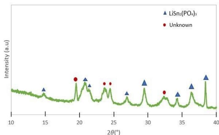
**Figure 5** X-ray diffraction pattern of the composite electrolytes sample.
