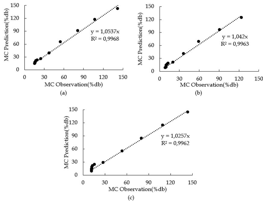
**Figure 3** Validation of the prediction model against observed biofoam moisture content using  $R^2$  values for: (a) mesh 60, (b) mesh 80, (c) mesh 100
