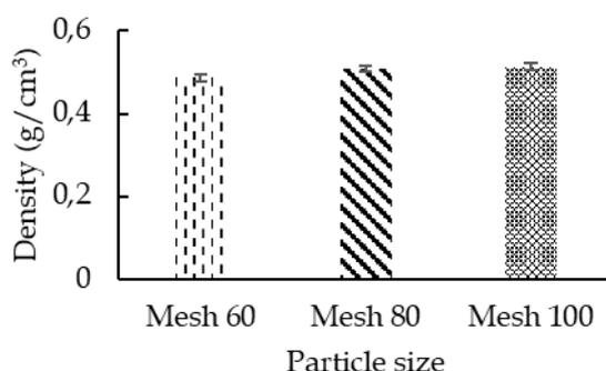
**Figure 5** The biofoam density at various particle sizes.
