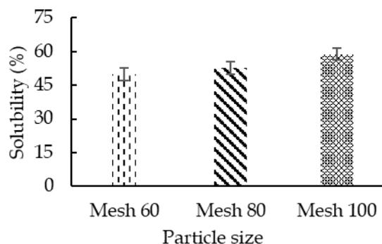
**Figure 9** The solubility of biofoam at various particle sizes.
