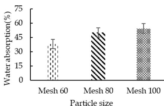
**Figure 8** The water absorption of biofoam at various particle sizes.
