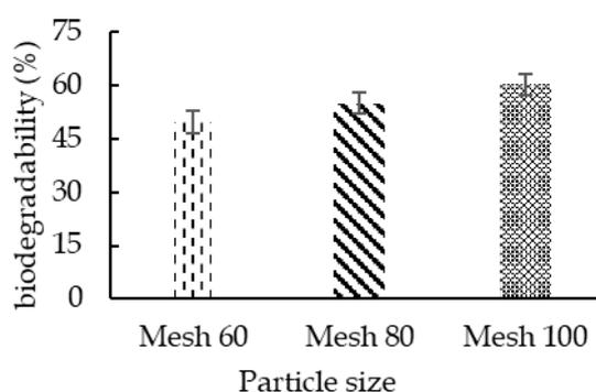
**Figure 7** The biodegradability of biofoam at various particle sizes.
