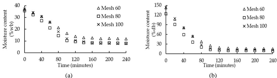
**Figure 1** Rate of change in moisture content during the drying process, (a) *wet* base, (b) *dry* base.
