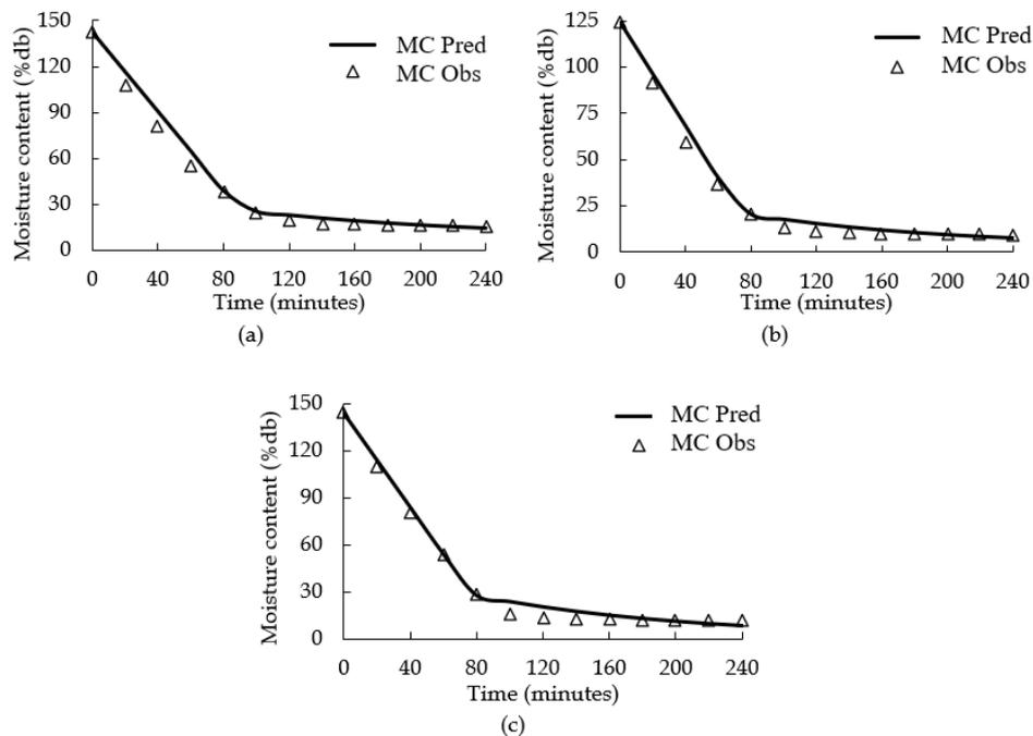
**Figure 2** Observed and predicted drying rate of biofoam during the drying process (a) mesh 60, (b) mesh 80, (c) mesh 100.
