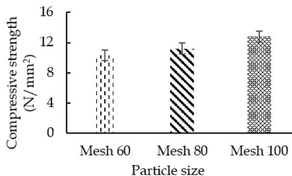
**Figure 6** The compressive strength of biofoam at various particle sizes.
