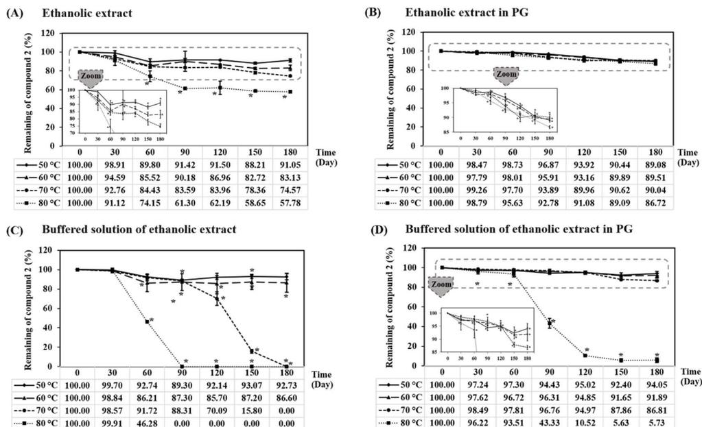
**Figure 4** The effect of temperature on the stability of **2** in (A) ethanolic extract (B) ethanolic extract in PG (C) buffered solution (pH 5.5) of ethanolic extract and (D) buffered solution (pH 5.5) of ethanolic extract in PG. (\* $p < 0.05$  against data of day 0).
