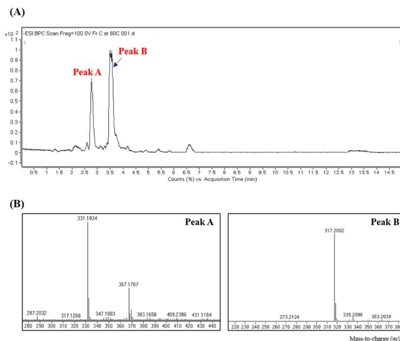
**Figure 6** The (A) baseline peak chromatogram (BPC) of sub-fraction C (10 mg/mL) from LC-MS and (B) mass fragmentation (in negative mode) of peaks A and B.
