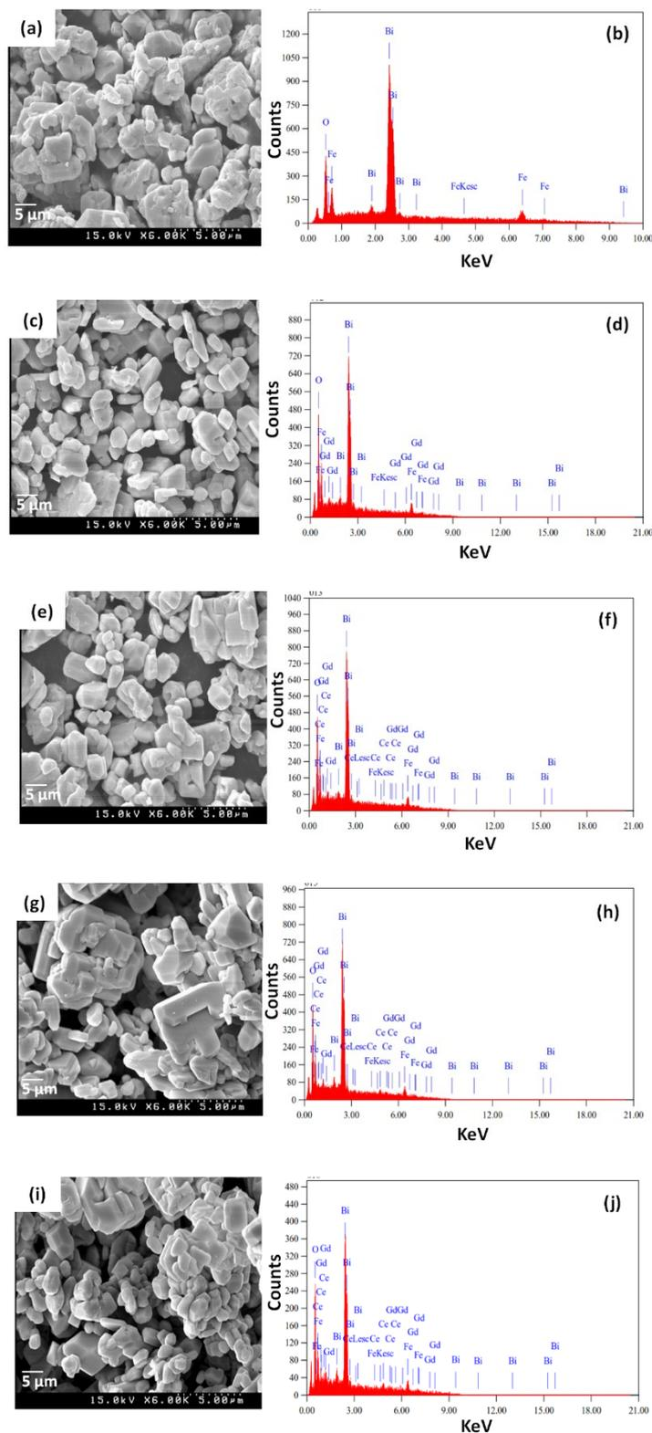
**Figure 2** The FE-SEM and EDAX images; (a-b) BFO, (c-d) BGF-1, (e-f) BGCF-1, (g-h) BGCF-2, and (i-j) BGCF-3 samples.
