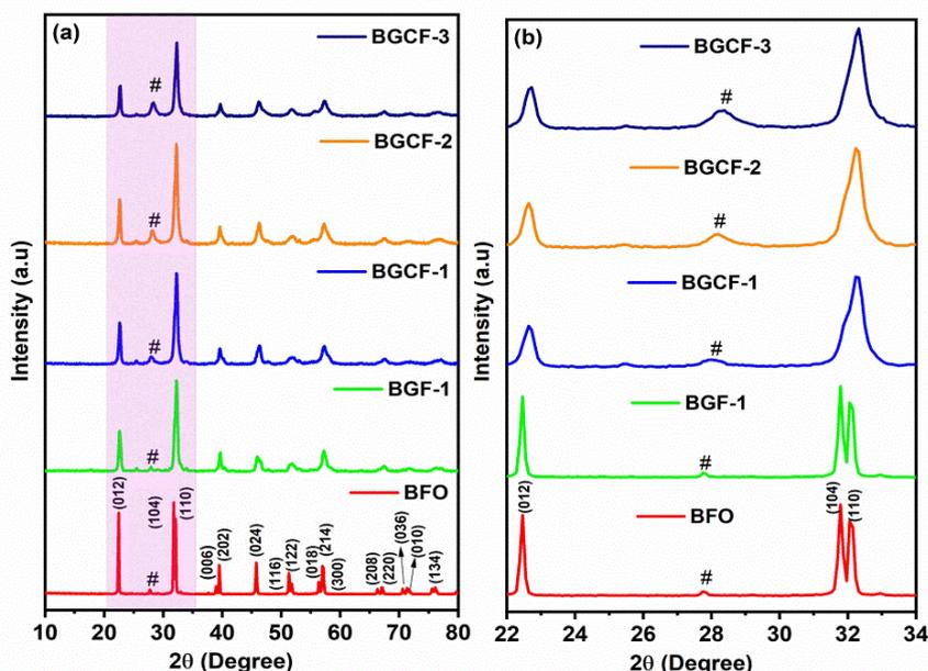
**Figure 1** XRD spectra of (a) BFO, BGF-1, BGCF-1, BGCF-2 and BGCF-3, (b) Magnified view of XRD pattern angle  $2\theta = 22$  to  $34^\circ$ , for BFO, BGF-1, BGCF-1, BGCF-2 and BGCF-3 samples.
