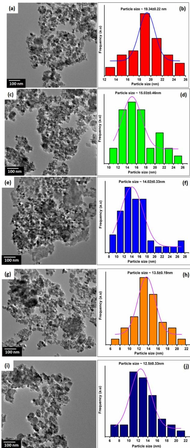
**Figure 3** TEM images and particle size distribution of (a-b) BFO, (c-d) BGF-1, (e-f) BGCF-1, (g-h) BGCF-2, and (i-j) BGCF-3 samples.
