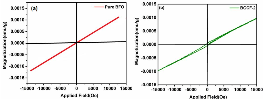
Figure 4 Room temperature M - H curves of (a) BFO, (b) BGCF-2 samples.
