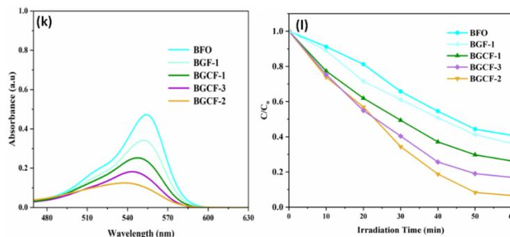
**Figures 5(k) - 5(l)** Champion results of absorption spectra and photocatalytic degradation efficiencies of RhB dye for BFO, BGF-1, BGCF-1, BGCF-2, and BGCF-3 samples.
