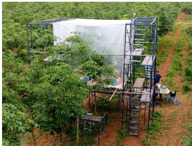
Figure 1 Overview of the large closed-chamber designed to field measure photosynthesis of whole tree crowns and pulse label trees with ^{13}\text{CO}_2 , installed on a rubber tree.
