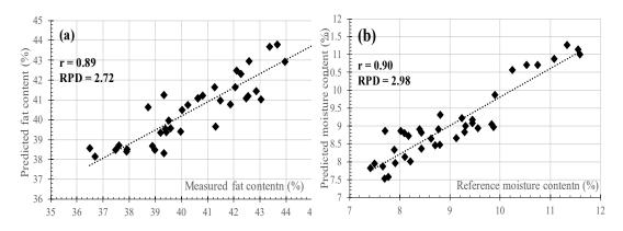
Figure 4 Validation performance for FC prediction (a) and MC prediction (b) using OSC spectra data.
