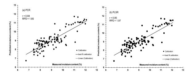
Figure 3 PCR and PLSR calibration to determine MC of the cocoa bean.
