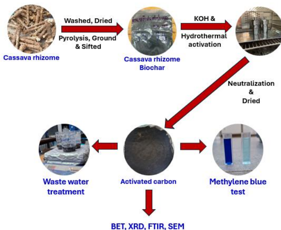
Figure 1 Schematic diagram of activated carbon preparation from cassava rhizome and its characterization and adsorption testing process.
