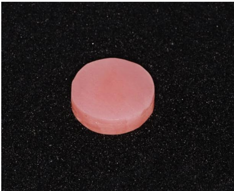
Figure 2 Acrylic surface after polishing.
